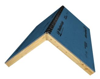
• 6" LP WeatherLogic® Seam & Flashing Tape is recommended. Center tape over ridge/hip. Fully adhere half of tape width to one side and then tightly wrap over ridge/hip to adhere tape to adjacent side.
